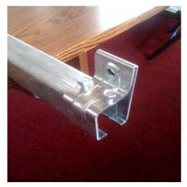
Ensure that at each end, the end bolt is secured stopping the truck from rolling beyond that point (see photo).
